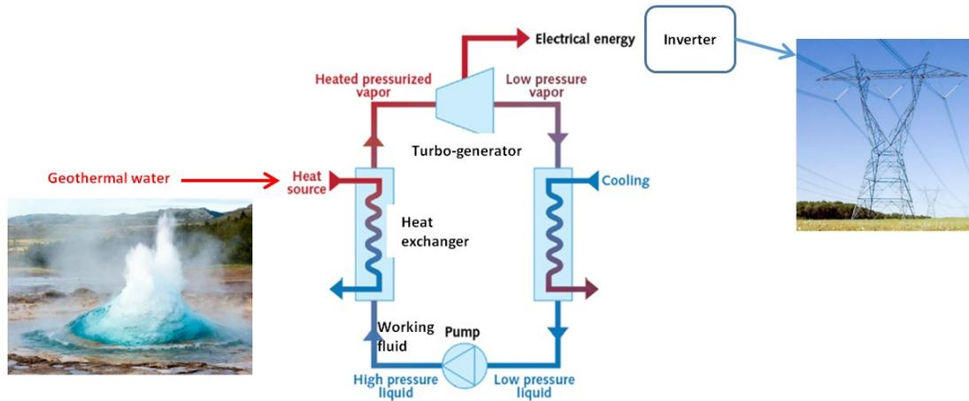
**Figure 5: ORC principle and application to geothermal heat source.**
