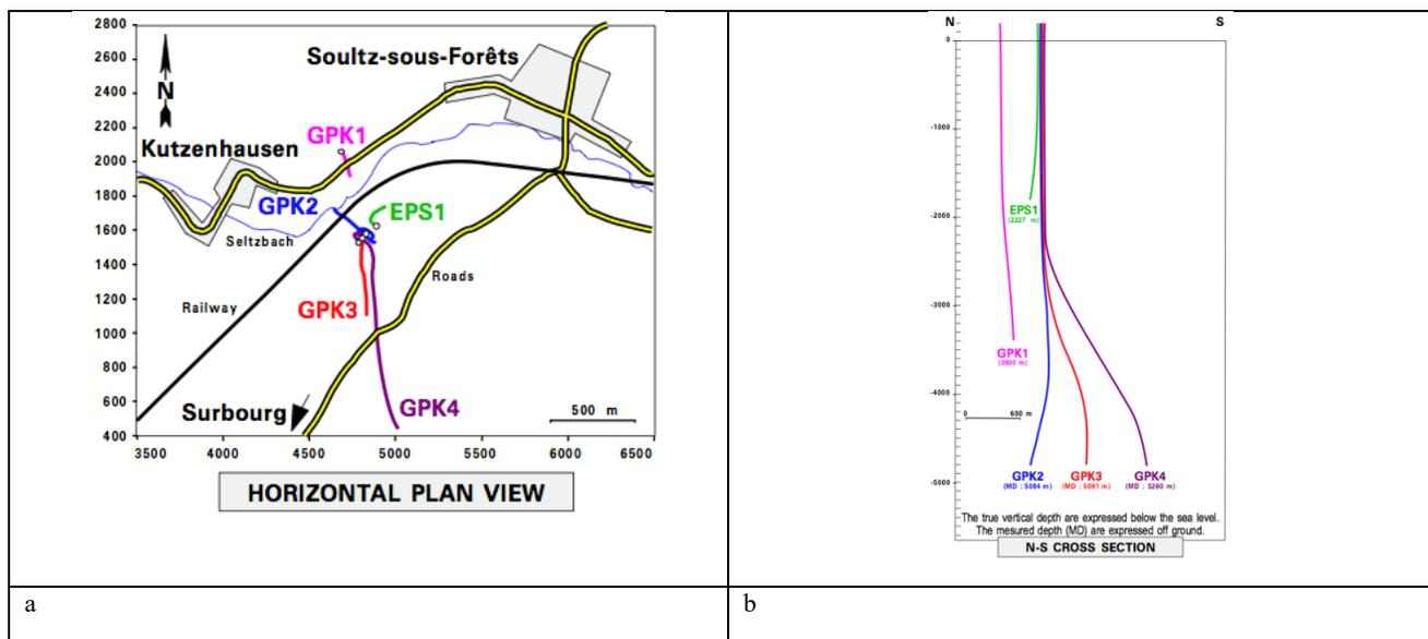
Figure 4: a) Horizontal map (a) and vertical cross-section (b) showing the well trajectories at the Soutz geothermal site.
