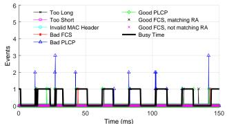
Time (ms) Fig. 5. Bursts of receiver events corresponding to the reception of Microwave interference.
