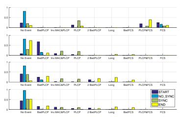
Fig. 8. Emission Probabilities of most significant observations for different experiments (from top to bottom: WiFi, ZigBee, LTE-U and Microwave).
