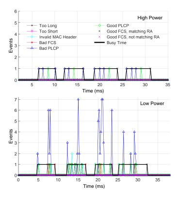
Fig. 4. Bursts of receiver events corresponding to the reception of ZigBee frames at high and low power.
