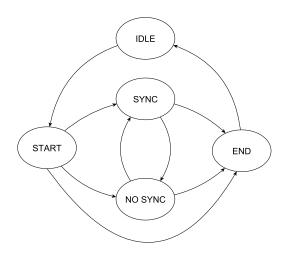
Fig. 7. Generalized state model of the receiver behavior: transition probabilities depend on the interference source.
