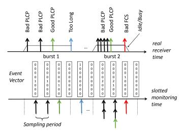
Fig. 3. Mapping between a real trace of receiver events and the time-slotted vectors generated by the monitoring process.
