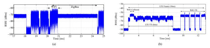
Fig. 1. Interference between technologies: temporal trace (RSSI samples) of WiFi-ZigBee (a) and WiFi-LTE collisions (b).
