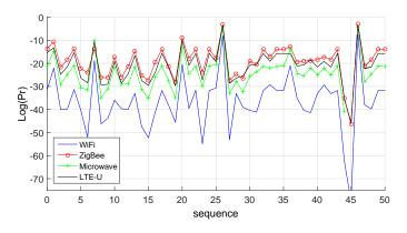
Fig. 10. Comparison between the burst-based receiver models for a sequence of error bursts due to ZigBee transmissions.
