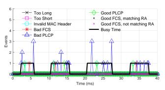
Fig. 6. Bursts of receiver events corresponding to the reception of LTE-U interference.
