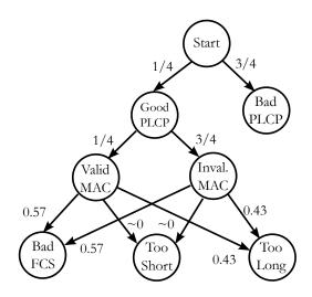
Fig. 2. Receiver events and relevant probabilities during cross-technology interference.
