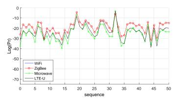
Fig. 9. Comparison between the time-based receiver models for a sequence of errors vectors due to ZigBee transmissions (N = 200).
