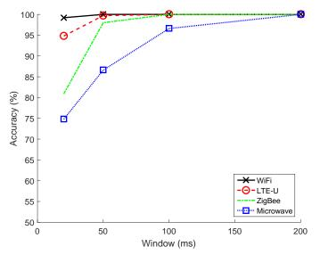
Fig. 11. Accuracy of the time-based receiver using different observation windows of 20, 50, 100 and 200 ms.
