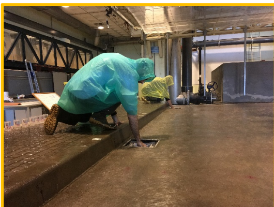
Figure 3. TSS samples in gully pots (left) and turbidity measuring point and samples in pipe system outlet (right).
