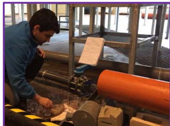
Figure 3. TSS samples in gully pots (left) and turbidity measuring point and samples in pipe system outlet (right).
