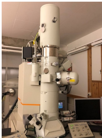
Figure 15. Photograph of the Transmission Electron Microscopy used in this chapter, JEOL JEM-2100F, with field emission gun (FEG), situated at the Arrhenius Laboratory, Stockholm University (Sept. 2018).
