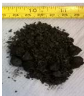
Figure 2. Char produced from pyrolysis (600 °C, 3 min SRT) of wheat straw pellets in the lab scale screw reactor at Aston University.
