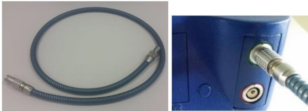
Figure 3: Transfer Line Connection to E-NOSE Device
