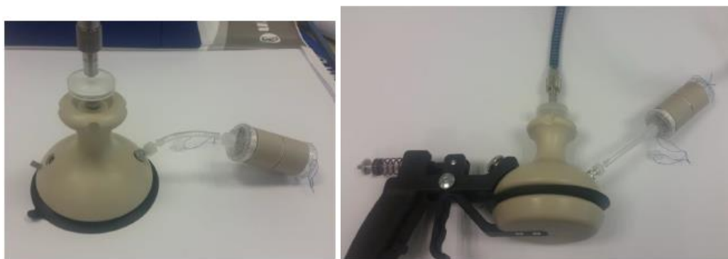
Figure 8: Air Sampler Connected to the Filter 2 (for surface measurement on the left and for leaves measurement on the right)
