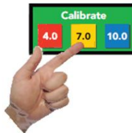
Figure 2: pH Calibration Buttons on the pH Transmitter Boards
