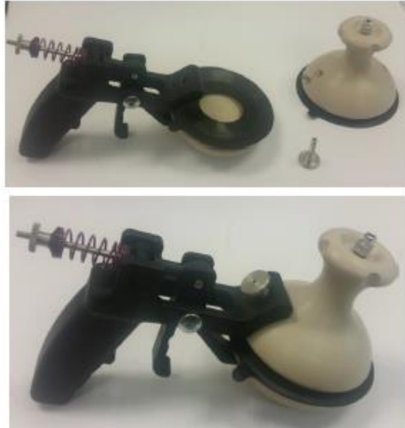
Figure 6: Configuration of the Air Sampler for Measurement on Plants
