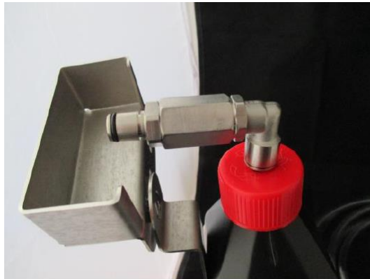
Figure 4: Suction Valve Installed on the bottle
