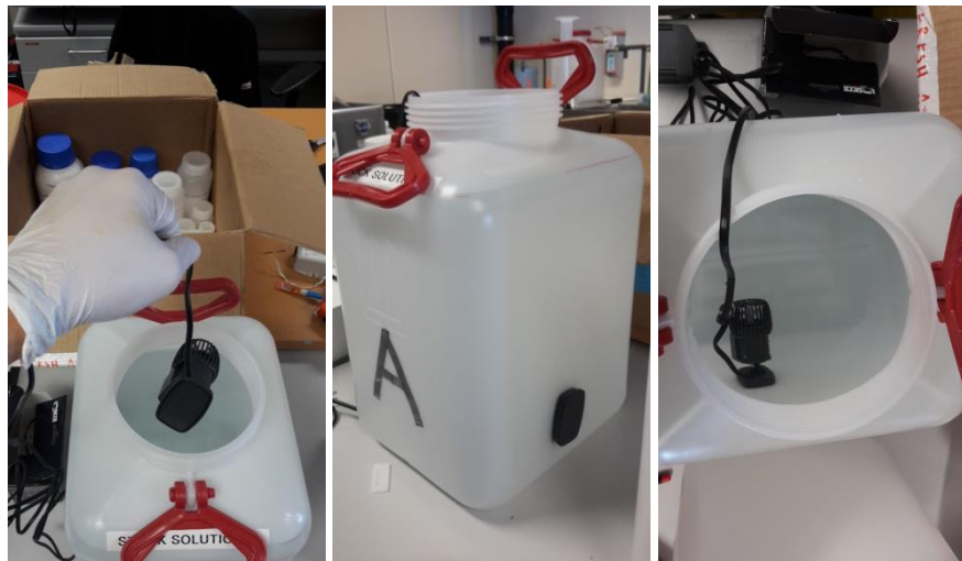
Figure 3: pump installation into the tank
