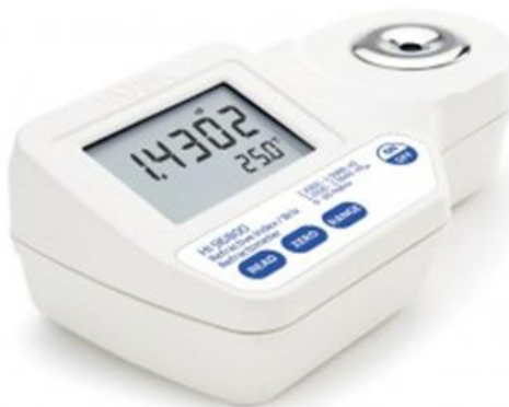
Figure 1: HANNA HI 96801 Refractometer
