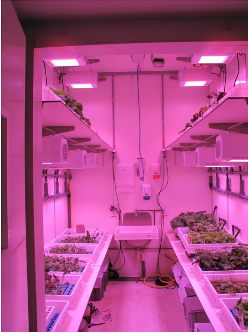
Picture 1: Climate chamber with 4 shelves and 12 lamps
