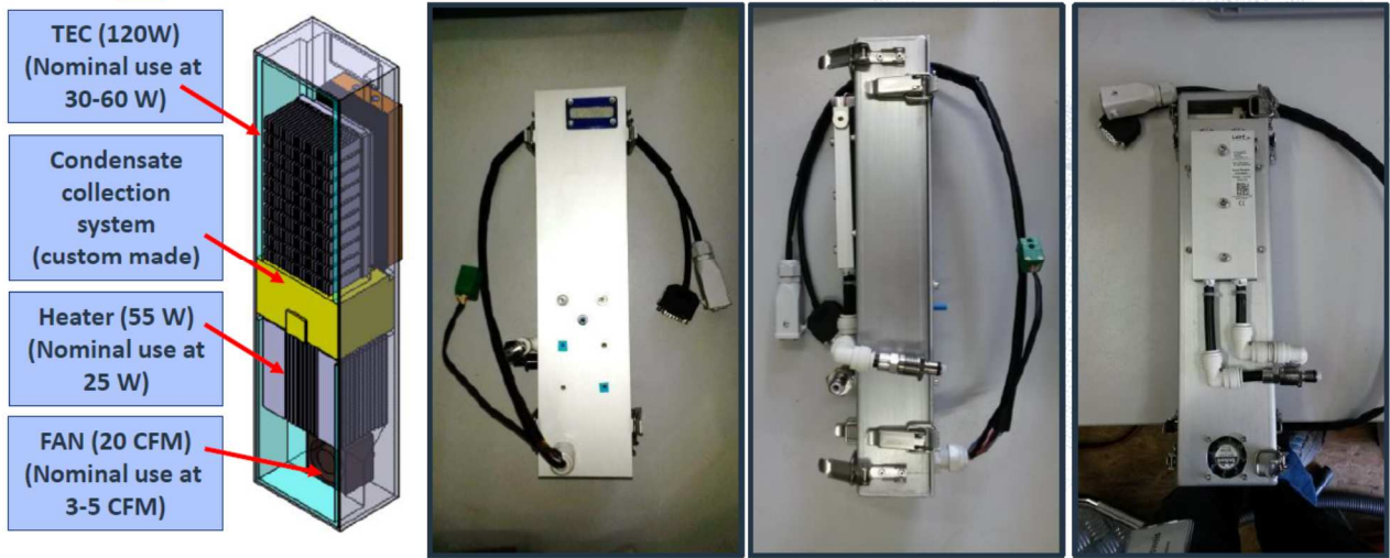
Figure 45: Temperature and Humidity Control Layer
