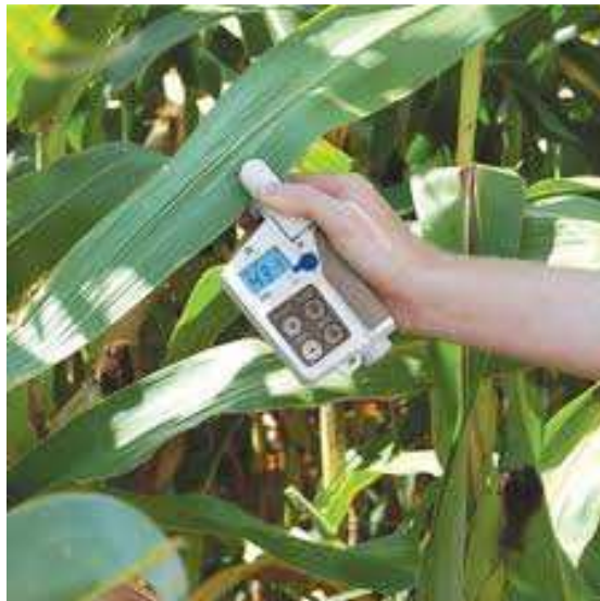
Figure 115: Use of the Chlorophyll SPAD Meter
