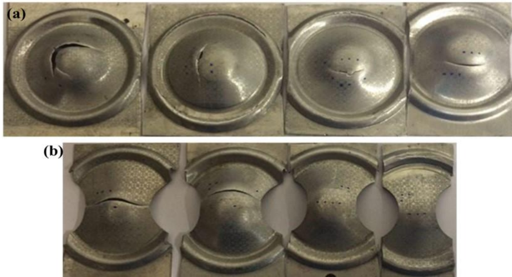
Figure 3: Typical deformed specimens for: (a) right side of FLD, and (b) left side of FLD
