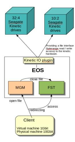
EOS storage servers (FST) provide a plug-in mechanism to replace IO to local attached disks with remote protocols. For the comunication between the EOS FST and the Kinetic Drives, a Kinetic IO plug-in has been developed.
