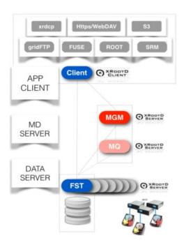
EOS is based on three components: management server (MGM), message queue (MQ) and file storage services (FST). All components are implemented as plug-ins for the *XRootD* storage server.
