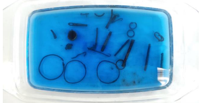
Figure 5: Treatment of rings, bracelets and fishing poles with alkaline Rochelle salt
