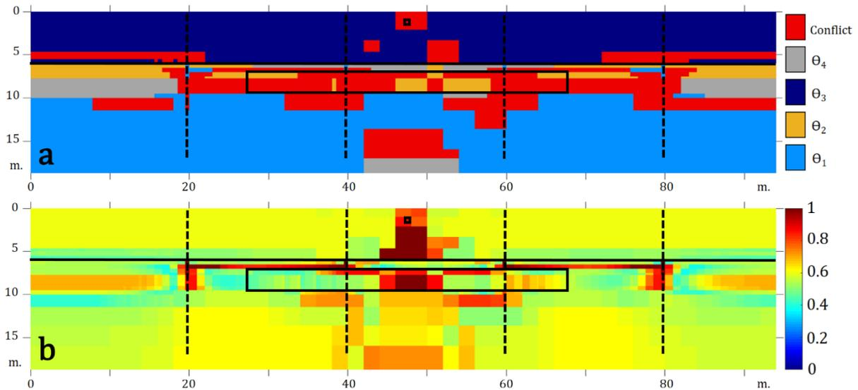
**Figure 2** Data merging with Smets' combination rule: *b*) represents the BBAs associated to the most plausible events presented in *a*). The black lines stand for the interfaces and the conductive anomaly fixed in the ER model (Figure 1.a) while the dashed lines stand for the boreholes position.
