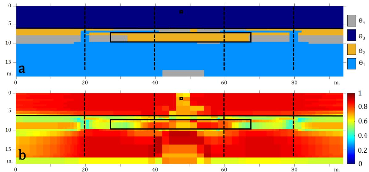
**Figure 3** Data merging with PCR5 normalization rule: *b*) represents the BBAs associated to the most plausible events presented in *a*). The black lines stand for the interfaces and the conductive anomaly fixed in the ER model (Figure 1.a) while the dashed lines stand for the boreholes position.
