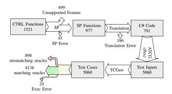
Fig. 2. Sankey diagram displaying the test generation and execution for the JCOP framework
