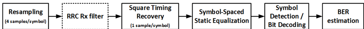
Figure 4. Receiver DSP implemented in MATLAB for the PAM-4 simulations. The RRC matched Rx filter was only used for the RRC pulse-shaped signal.
