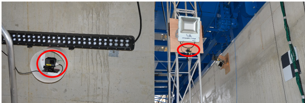
Figure 3-10: GoPro camera from side wall (left) and attached to scaffold structure (right) below the light sources
