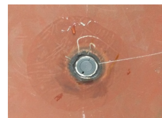
Figure 3-11: Void-fraction meter flash mounted in steel wall
