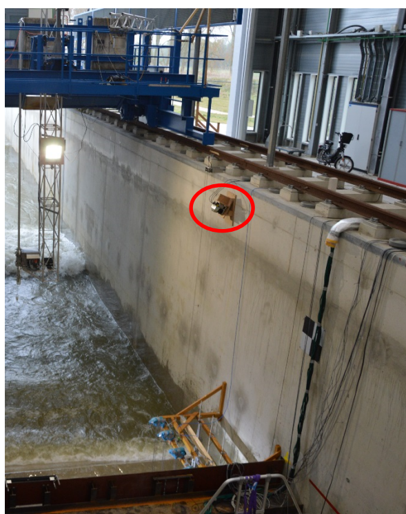
Figure 3-12: SICK laser profiler attached at the upper edge of the flume wall
