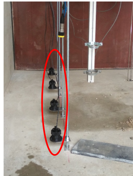
Figure 3-8: 4 Airmar paddle wheels attached to M10 screw
