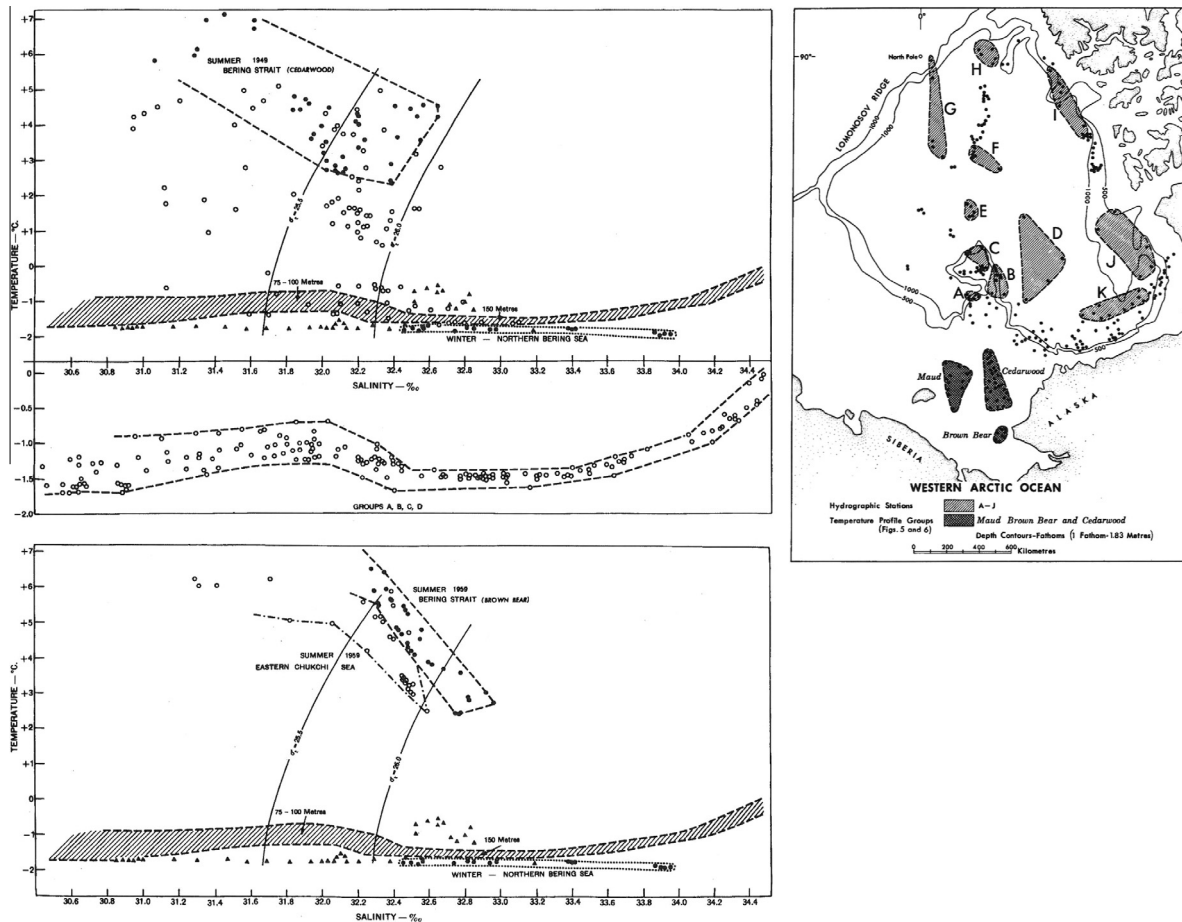
Fig. 5. TS characteristics of the upper layers in the southern Canada Basin and in the Bering Sea, Bering Strait and the Chukchi Sea showing the subsurface temperature maximum of the Bering Strait Summer Water (BSSW) and the temperature minimum of the Bering Strait Winter Water (BSWW). The map indicates the positions of the stations (from Coachman and Barnes, 1961 ).
