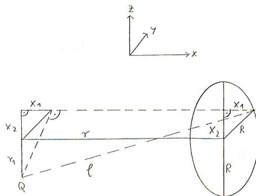
$Q$ = point light source (with luminous intensity  $I$ ), that is shifted with  $r_1$  from the coordinate origin.
