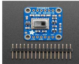
FIGURE 3.1: THERMAL SENSOR AMG 8833
