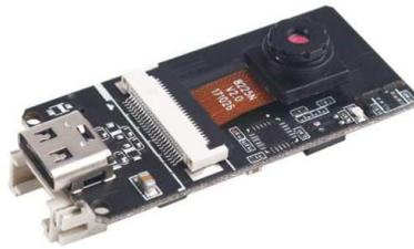
FIGURE 3.6: OPTICAL CAMERA ESP32
