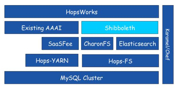
Figure 3. BiobankCloud Architecture with Added support for Shibboleth
