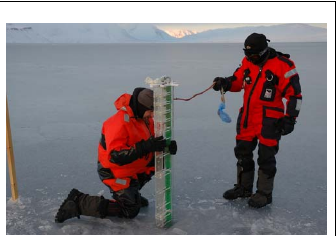
Deploying a newly developed instrument to measure sea-ice salinity in situ, which informs ongoing modeling activities to better understand the exchange of salt between sea ice and the underlying ocean. Photo: MPI-M
