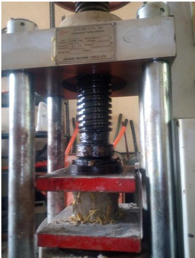
**Figure 1.** Sandcrete block undergoing compressive test.
