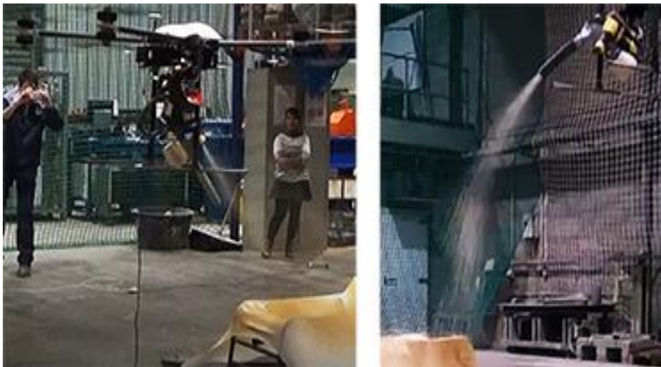
Figure. 1. Left: Drone spraying the clay + water mix. Right: Drone spraying a clay mix containing plaster.
