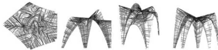
Figure 7. Karamba structure analysis of case study one from the AA showing the stress lines of the shell structure. of the shell structure.
