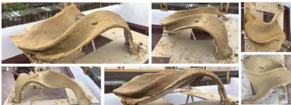
Figure 12. Failed experiment of a shell collapsed when applying different layers of clay mix, because the initial geometry was not matching the viable thresholds.
