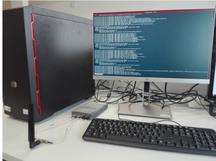
Figure 40: OAI lab hardware components (eNB, USRP, antenna)
