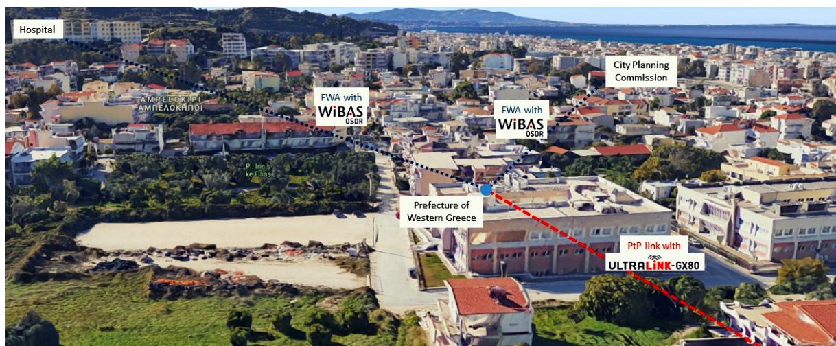
Figure 28: Illustration from Radio Planning for FWA Network at Patras Facility-site
