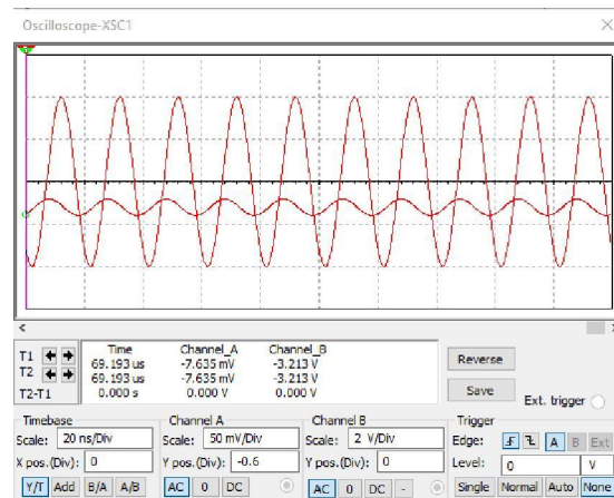
Fig.3. Output result of notch filter using THS3202 IC
