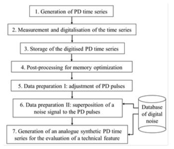
Fig. 1. Flow diagram of the procedure applied for the realization of the reference PD time series.
