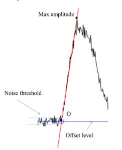
Fig. 4. Detection of the PD pulses and determination of their origin for the final digitalisation.
