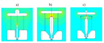
Fig. 3. Layout of the test cells and electrical field distribution calculated by means of FEMM. a) Corona effect in air, b) internal defect in polyethylene and c) surface defect in glass.
