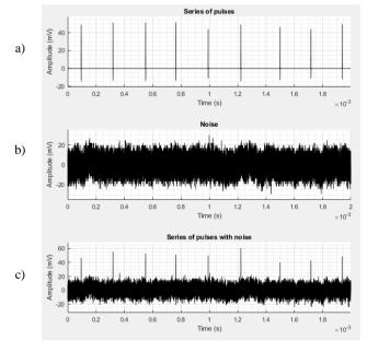
Fig. 6. Synthetic generation of analogue PD time series. a) Corona effect, b) pink noise and c) simultaneous generation of the corona effect and the pink noise.
