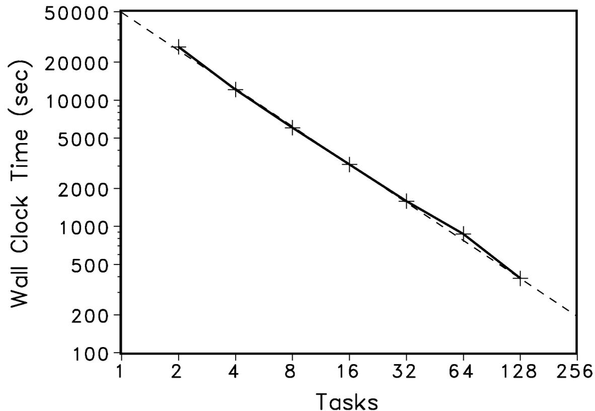
Run time on a 3 GHz Xeon Intel cluster with Infiniband network.
