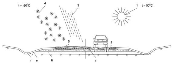
Figure 1. External impacts on road coverage. a - road pavement; b - earth bed; c - railroad slope; d - road ditch 1 - temperature, t=+50°...-20°C; 2 - load from automobile transport, P; 3 - rain; 4 - snow; 5 - salt ingredients.
