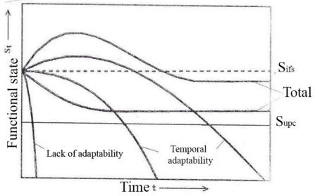
**Figure 2.** Variants of the trajectories of the functional state S1 of concrete in time t in the operational environment. S<sub>ifs</sub> - the initial functional state, S<sub>upc</sub> - ultimate permissible state. According to research of V.L. Chernyavsky [10].
