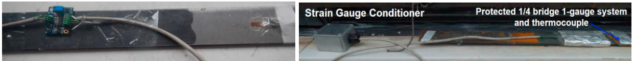
Fig. 6. Quarter bridge SG configuration: 1 active-gauge 3-wire system in lab (left image) and in the field (right image).
