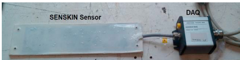
Fig. 1. View of the novel SENSKIN sensor accompanied by its Data Acquisition Unit (DAQ).
