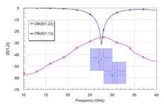
Fig. 7 Dual Polarization antenna array. Return loss and mutual coupling between antenna elements (dense array)
