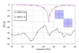
Fig. 6 Dual Polarization antenna array. Return loss and mutual coupling between antenna elements
