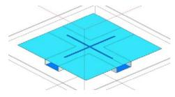
Fig. 1 Dual Polarization antenna design
