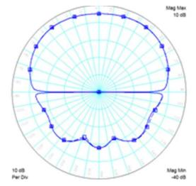
Fig. 5 Dual Polarization antenna for 28 GHz. Radiation patter of the antenna (solid line –XZ plane and dashed line – YZ plane). The directivity is 5.0dBi
