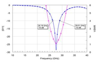
Fig. 4 Dual Polarization antenna for 28 GHz. Return loss and VSWR versus frequency
