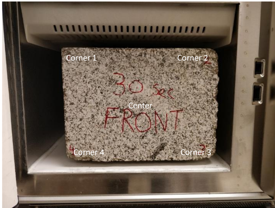
Figure 16 Temperature reading locations on the rock kept inside the microwave cavity.
