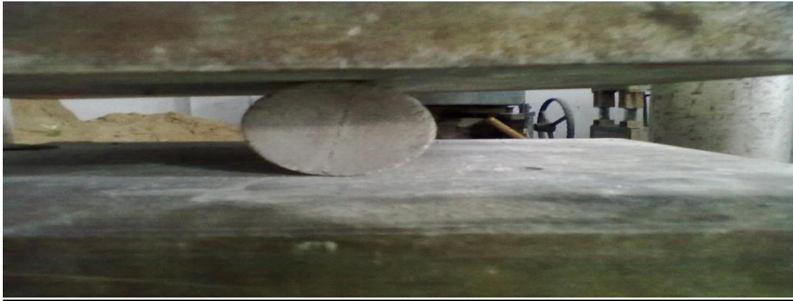
Figure 6: Split Tensile Test in CTM.
