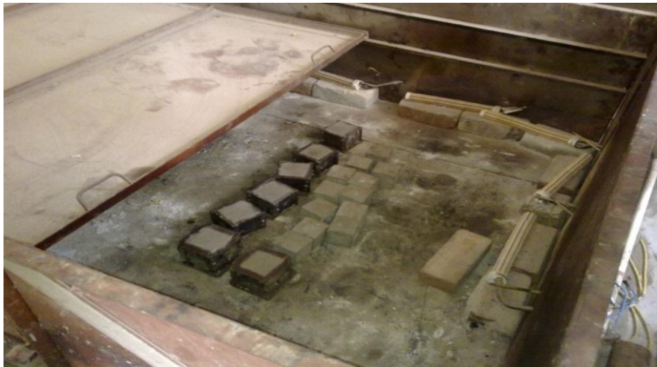
Figure 2: Heat curing Chamber.
