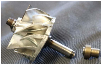
Compressor failure after 200 h of testing: broken impeller shaft
