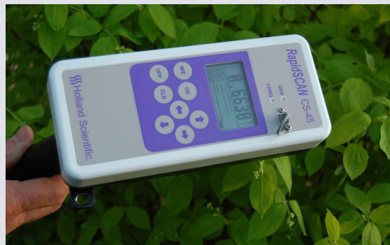
Figure 8: Crop Circle RapidSCAN AC-45 handheld reflectance sensor
