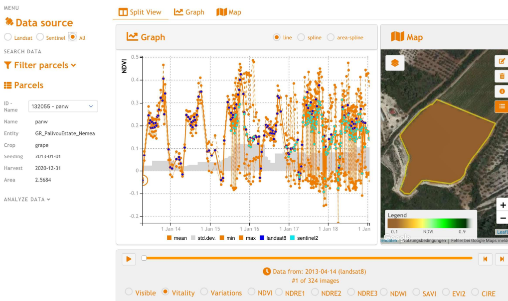
Figure 28: A combined Landsat-8 & Sentinel-2 NDVI time series for 2013 - 2019 over a parcel of the Palivou estate in Greece, visualized in a data analysis and review client
