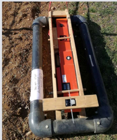
Figure4: EM38-MK2 (left) and Archer Data logger (right)
