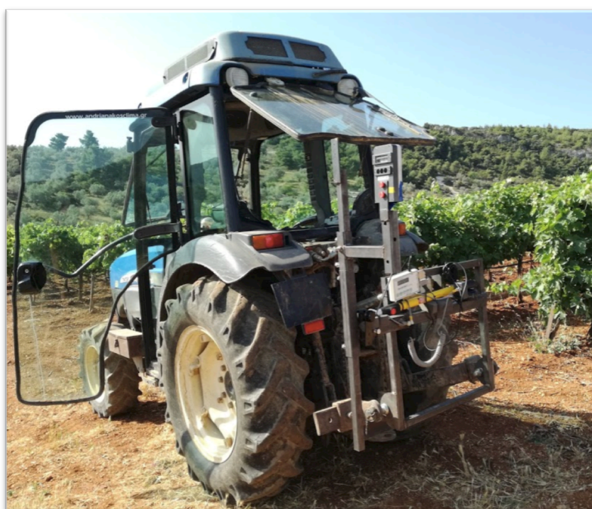
Figure 8: Both canopy sensors mounted on a tractor
