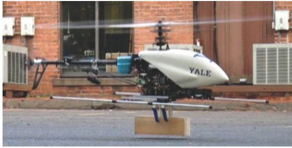
Fig. 3. Example of a flying hand, in particular the Yale Aerial Manipulator capturing a block in hover (picture taken from [45]).
