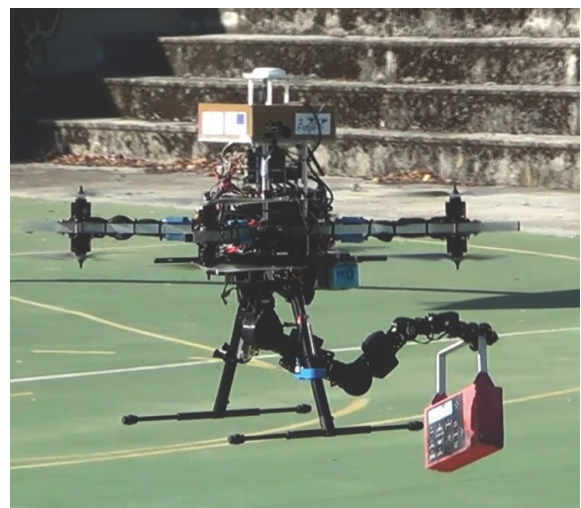
Fig. 5. Unmanned aerial manipulator composed by a multirotor, an eight rotor aircraft in coaxial configuration, equipped by a 7-DoF servo-driven manipulator, developed at University of Seville within the ARCAS project [71]. More details about this UAM can be found in [74].
