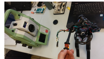
Fig. 6. Test-bench with laser system for measuring the accuracy of the docking tool.
