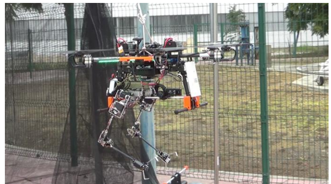
Figure 1. Aerial manipulation system consisting of the anthropomorphic compliant dual arm manipulator integrated in a hexarotor platform. The rope above the UAV was used for safety but did not have a significant influence in the dynamic behavior.
