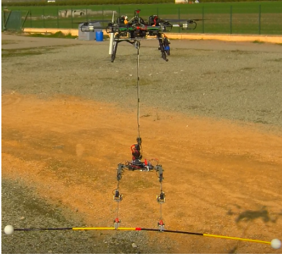
Fig. 1. Aerial robotic system with two arms for long-reach manipulation.
