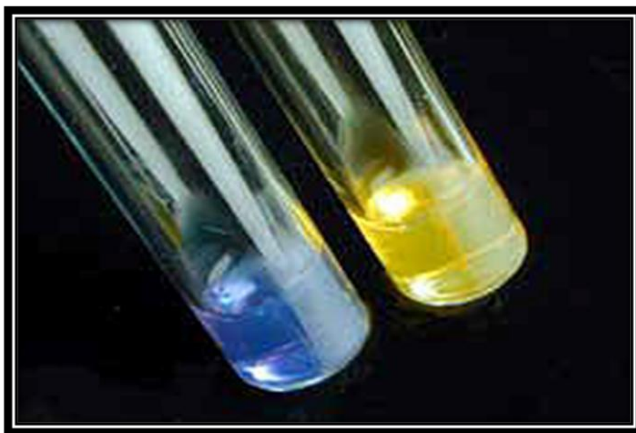
Fig.5- Blue color indicates negative test whereas Yellow color indicates positive test.
