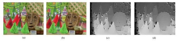
Fig 6. Initial disparity estimation results of Cones image pair (a) left image (b) right image (c) initial disparity map generated by SAD (d) initial disparity map generated by proposed approach.
