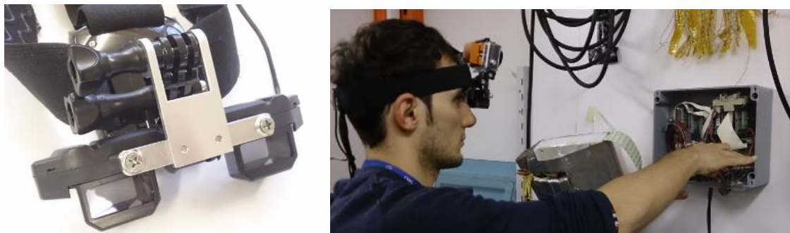
Figure 8: The HMD system. The display part without the tracking component (left), the system worn by a user with a tracking camera & an inertial measurement unit integrated (right)
