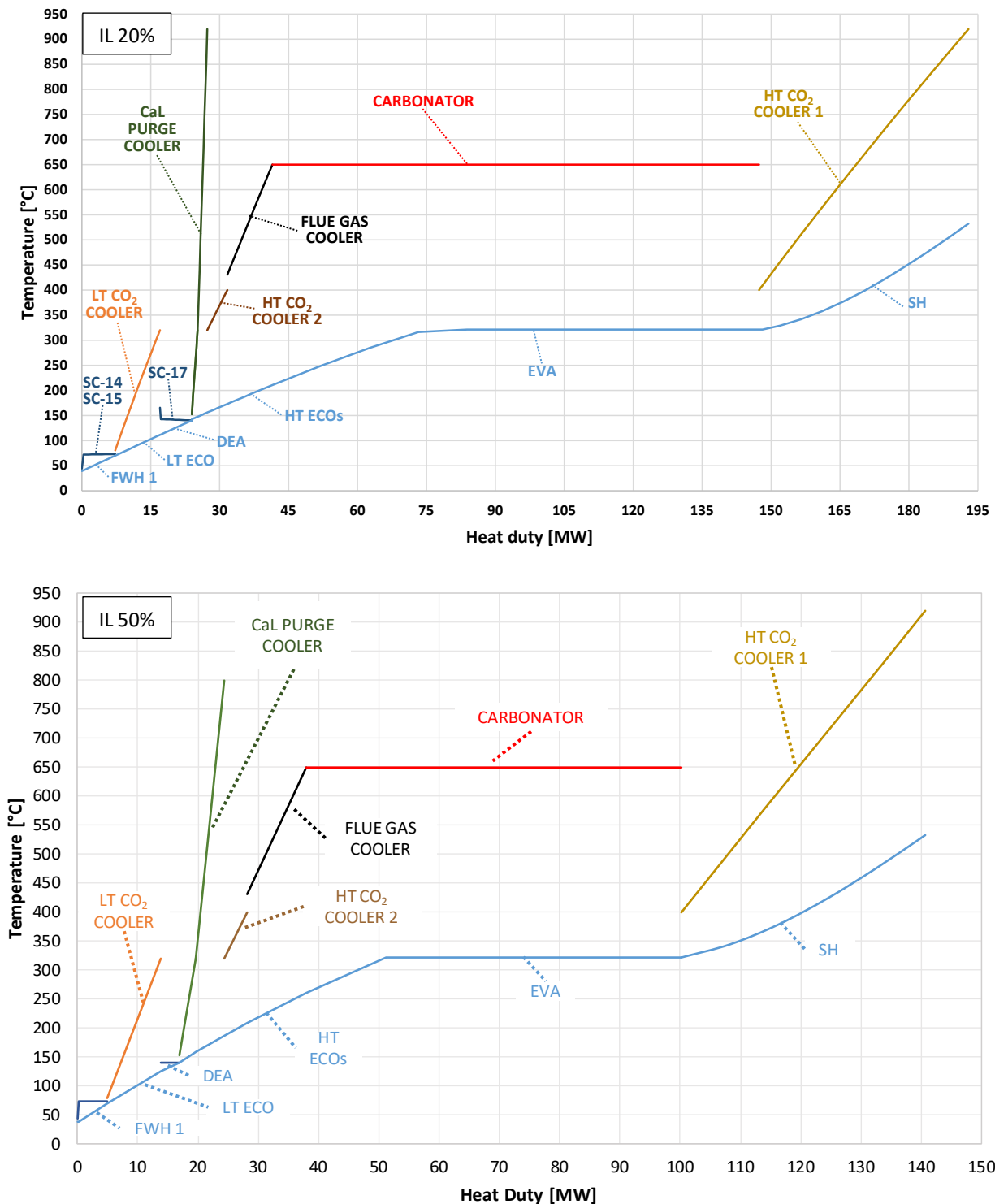
Figure 2.4: T-Q cumulative diagram for the heat recovered from CaL streams for the Tail End CaL configuration with IL 20% (top) and IL 50% (bottom)
