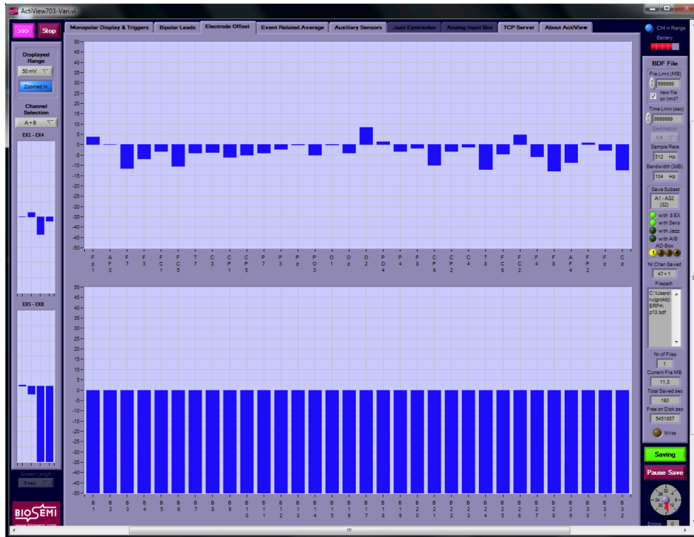
Figure 29: ActiView window showing electrode offset. Full blue bars represent unconnected channels.
