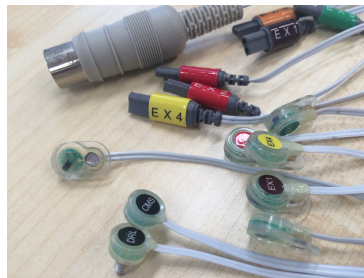
Figure 25: Flat electrodes and CMS-DRL cable
