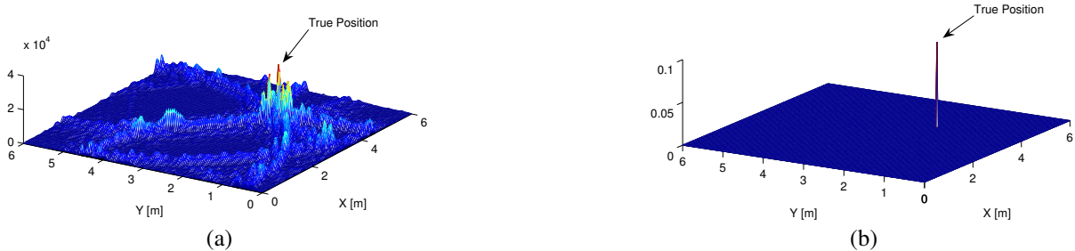
Fig. 1. Target localization results evaluated in IEEE 802.15.4a CM7 Industrial LOS, SNR=4dB, obtained by (a) conventional DPE with \rho = 1 and (b) CS-based DPE with \rho = 0.25 .
