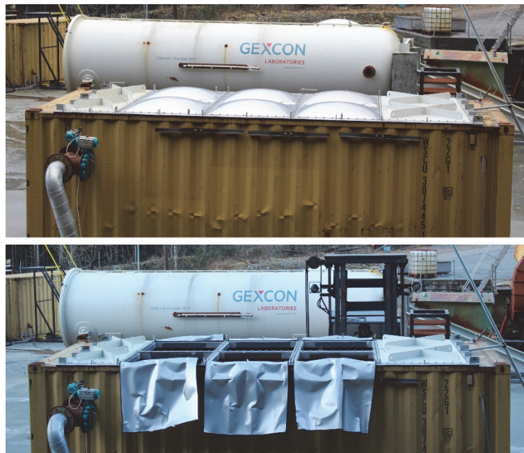
Figure 6: Container with six commercial vent panels before and after a test.
