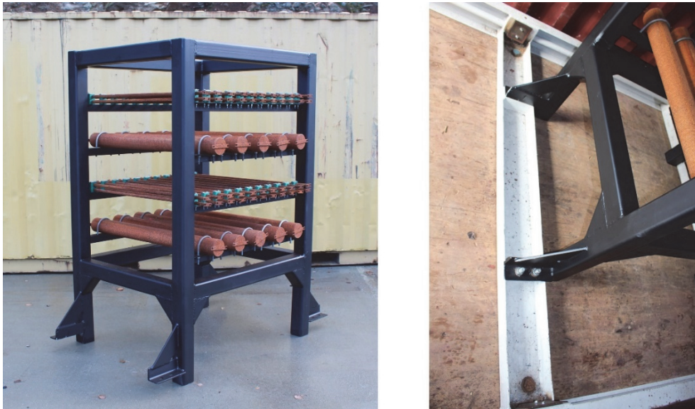
Figure 7: Pipe rack (left) and brackets fixed to frame inside container (right).
