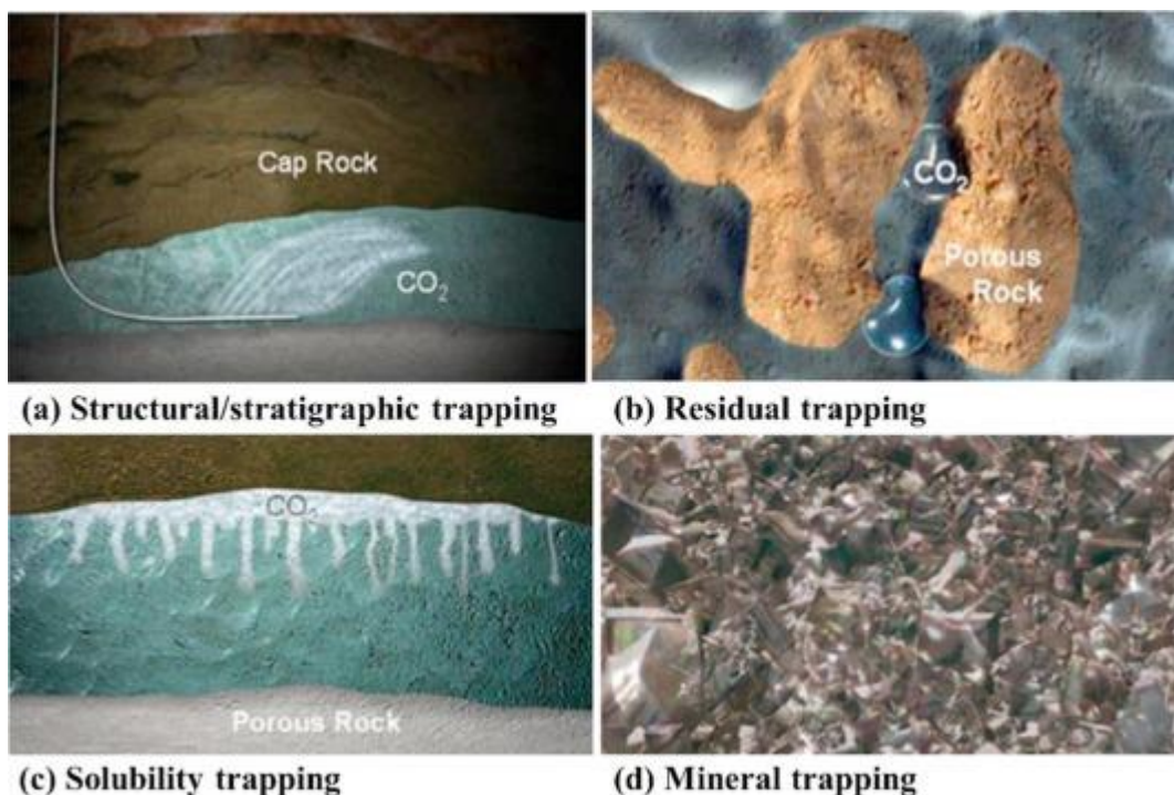
Figure 12-2: The four main CO 2 trapping mechanisms. Source: [173]
