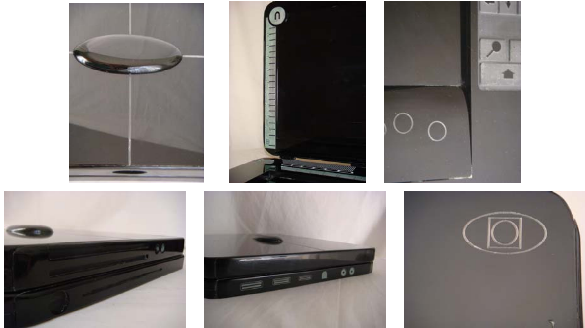
Figure10: Most important tactile signs on various areas of the LTB
