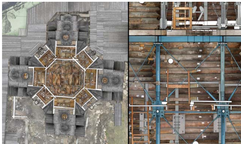
Fig.17 Post production results of the case study of the Church of the Transfiguration. In order to understand the wooden structure nine floor plans and four sections were produced by elaborating orthophotos by using the photo documentation elaborated on field and detailed technical drawings
