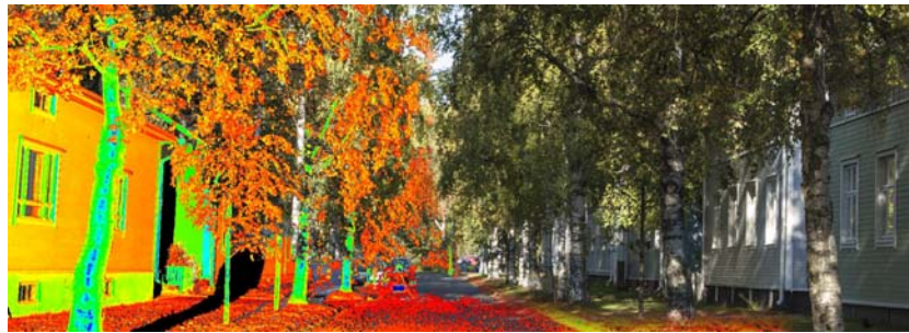
Fig.6 The study case of the historic district of Raksila in Oulu, Finland. Laser scanning survey, analysis and documentation of the street facades with census activity of the architecture and its environment. Analysis and results included in the report Özlem Özer-Kemppainen (a cura di) "Historiallisen Kaupunkimiljöön Suojeluatlas: Oulun Raksila" (English translation: Historical Urban Environment Protection Class: Raksila in Oulu) Oulun Yliopisto: Oulu. 2017
