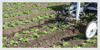
**Figure 2:** Illustrates robotic weeder is operating in a field near Santa Maria, CA. Image Credit: Image courtesy of Steven Fennimore [2].
