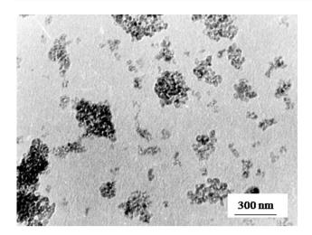
Fig. 1 TEM image of ZrO<sub>2</sub>-3 mol% Y<sub>2</sub>O<sub>3</sub>, 400 °C, 2 h nanopowder
