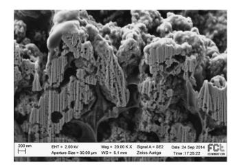
Fig.3 SEM cross-sectional image of deposited  $\rm ZrO_2\!\!-\!\!3$  mol%  $\rm Y_2O_3/$  PVA film
