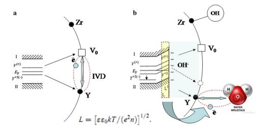
**Fig. 6** Schematic representation of the adsorption mechanism of electron emission. System before (**a**) and after (**b**) adsorption of water molecules, where: I—conduction band, II—valence band, OH<sup>-</sup>—negatively charged hydroxyl groups,  $Y^{+3(-)}$ —the acceptor level corresponding to the surface Y atom, V<sup>+</sup>—is the donor level corresponding to the oxygen vacancy  $V_a$ , *L*—the length of the region where
