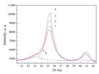
**Fig. 5** XRD spectra of the  $ZrO_2$ -3 mol%  $Y_2O_3$  nanopowder, where 1—after saturation under humid environment at 300K for 24 h; 2—after drying at of 400 K for 30 min; 3—after drying at a temperature of 500 K for 30 min; 4—after cooling from 500 to 320 K under vacuum for 24 h; 5 and 6 are the peaks of the monoclinic phase, extracted from spectra 1 and 2
